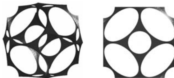
Fig. 8. Single cell model of open cell foam taken into considerations
